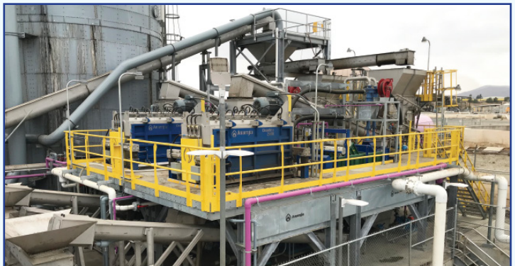
An organics polishing system similar to this one will be installed at VWRA.
