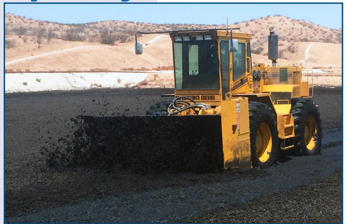
The new Brown Bear 400 being used to mix biosolids on our solar drying beds.
