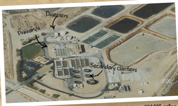
Aerial shot of the plant in 2000. The plant featured three 330,000 gallon digesters, four primary clarifiers and 6 secondary clarifiers. In those days, we used chlorine to disinfect the treated water. Today, we use powerful ultra violet lights in our disinfection process.
