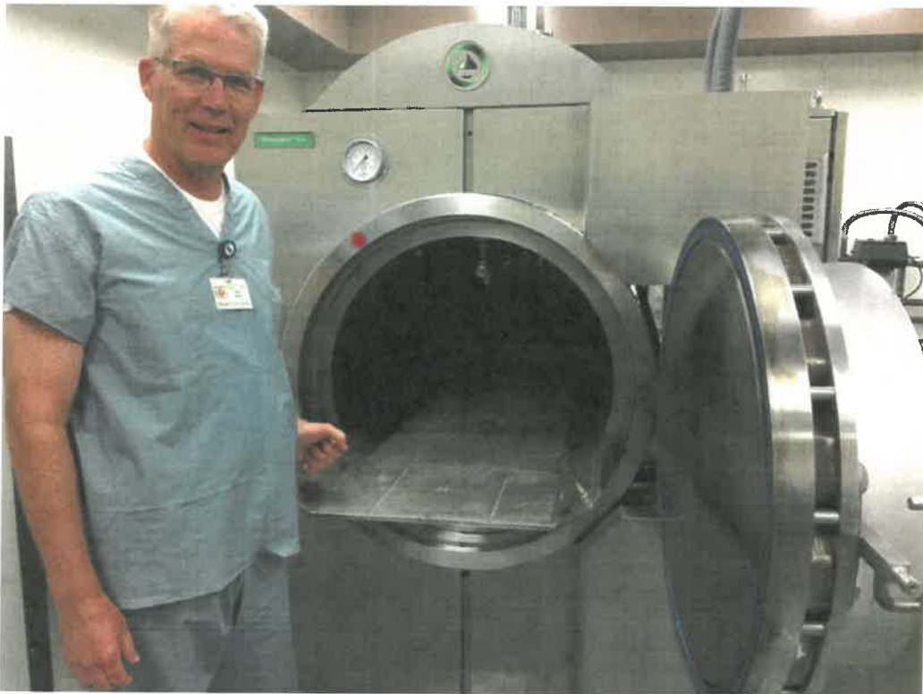
UCLA’s Dean Fisher opens an alkaline hydrolysis machine that can dissolve bodies. ( Lesley McClurg/KQED )
